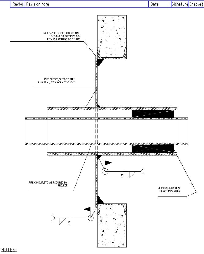
ALL WELDING & PLATE WINDOW & PIPE SLEEVE FIT UP TO BE SUPPLIED BY CLIENT.
